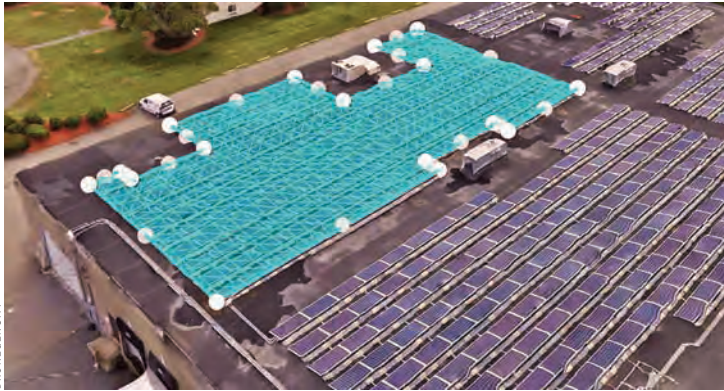
The combination of drone imagery with artificial intelligence and data analytics can be used to calculate capacity for solar arrays.
